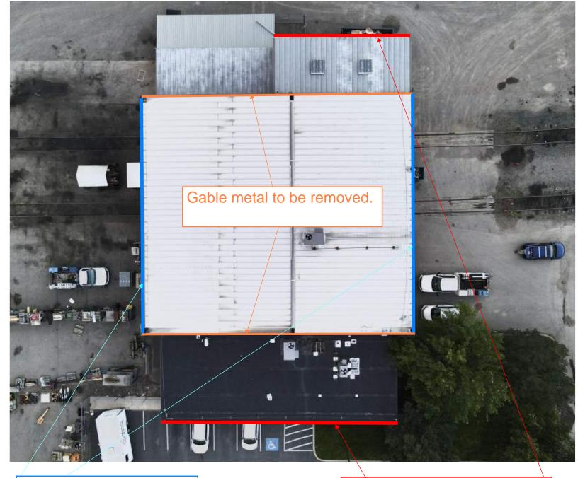
Edge to be cut back and new gutter and downspouts.
